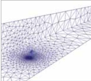
▶ A multi-scale simulation of a marine outfall discharging dense desalination plant effluent. The unstructured adapted mesh includes elements whose edge lengths vary by a factor of 10,000.
